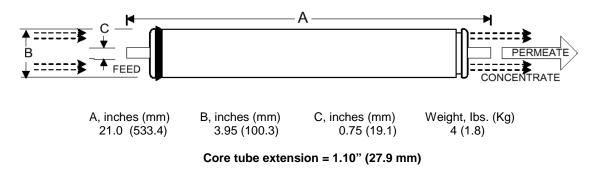
Notice: Minimum permeate flow for individual elements is 15 percent below listed flow. All membrane elements are supplied with a brine seal and o-rings. Most elements are packaged dry, sealed in a polyethylene bags, and shipped in a cardboard box. Some elements are sealed in polyethylene bags containing less than 1.0% sodium meta-bisulfite solution and shipped in a cardboard box.
